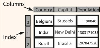
A two-dimensional labeled data structure with columns of potentially different types
